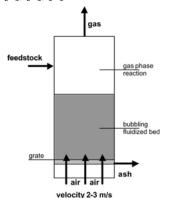
Fig. 1. Bubbling fluidised bed gasifier [7]
