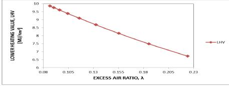
Fig. 5. The variation of lower heating value of syngas with the excess air ratio
