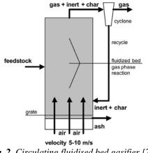
Fig. 2. Circulating fluidised bed gasifier [7]
