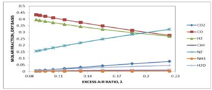
Fig. 3. The influence of the excess air ratio on the syngas composition for sunflower husk
