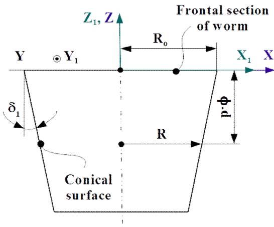
Fig. 6. Axial section of conical surface; reference systems
