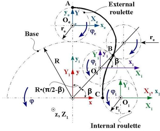
**Fig. 5.** Cycloid profile of worm. Reference system
